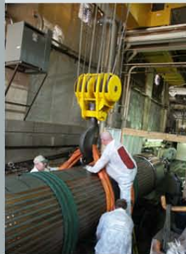
Rotor testing in the largest balance pit in North America, located in Columbus, Ohio.
